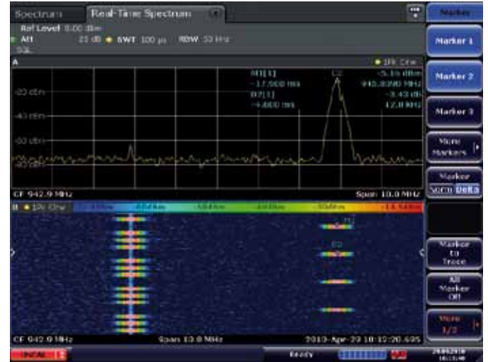
Spectrum and spectrogram of GSM signals on different frequency bands. Markers are used to measure a frame length of 4.6 ms.
