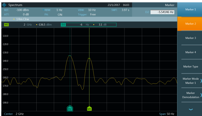
R&S®FPC-B22: high sensitivity with 1 Hz resolution bandwidth.
